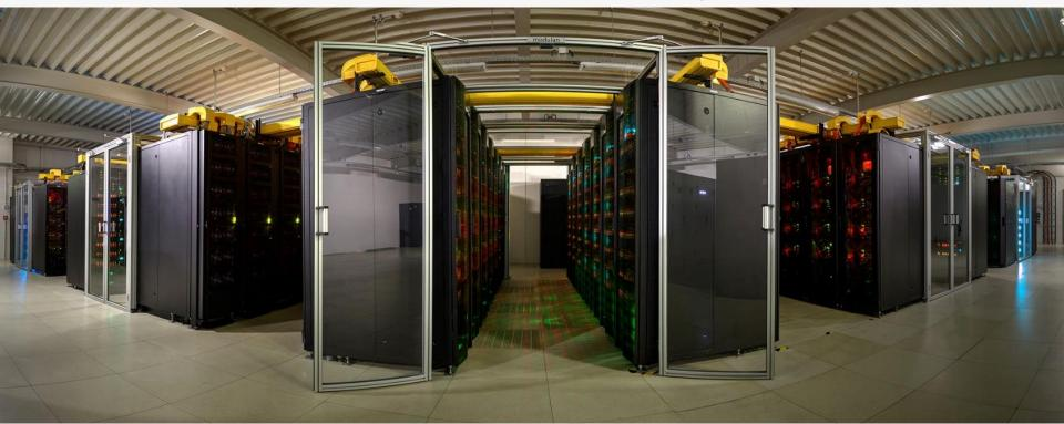
bullx DLC 720, 3,500+ nodes, 100,000+ cores, Haswell/Broadwell, 3.6 PFLOPS 240 TB main memory, 54 PB disk storage, 450 GB/s mem-disk rate, FDR network 21 GPU nodes for visualization hot liquid cooling with high efficiency
