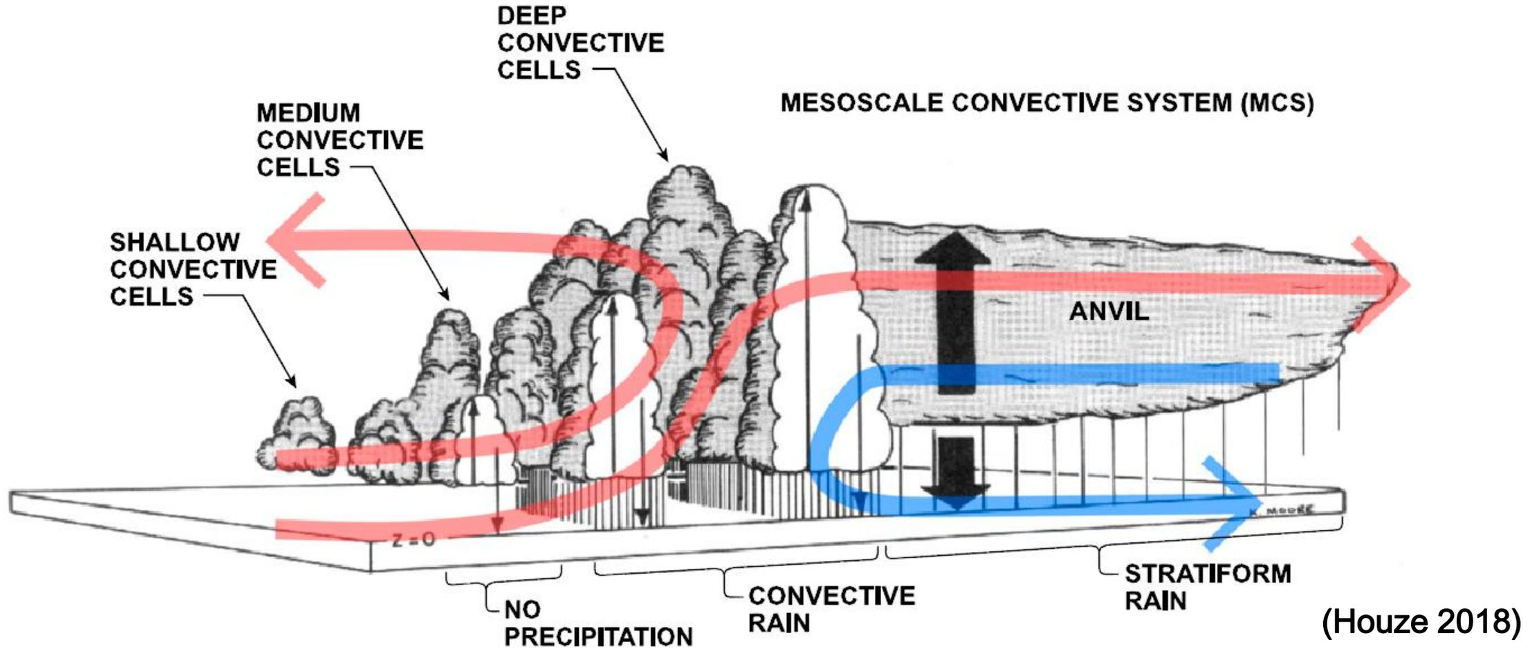
FIG. 17-52. Overlay of a convective cloud population and superimposed layered overturning. Adapted from Houze et al. (1980) and Moncrieff et al. (2017).
