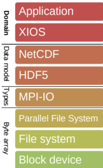
I/O path for an MPI-parallel application. HDF5 can be replaced with ESDM.
