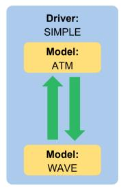
Coupled system with a Driver, two Model components, and two Connectors
