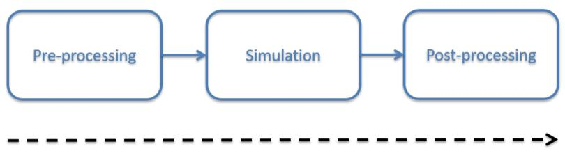
Critical path = Pre-processing + Simulation + Post-processing
